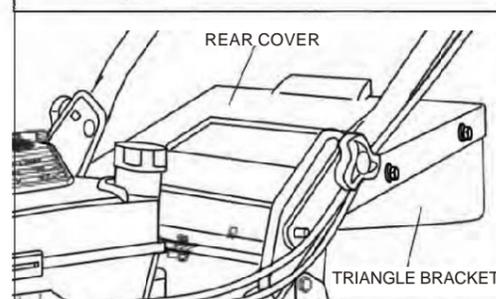
**CAUTION:** Do not run your lawn mower without rear door closed or approved grass catcher in place. Never attempt to operate the lawn mower with the rear door removed or propped open.
