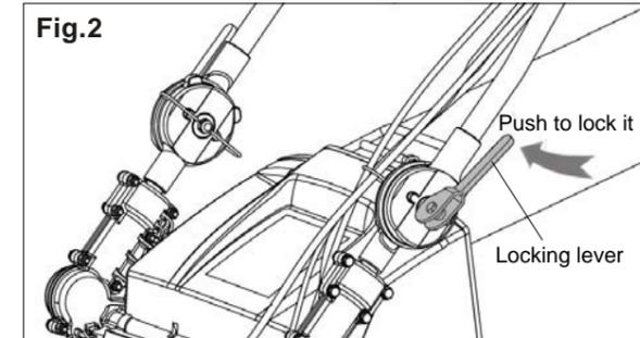
**CAUTION:** Unfold the handle carefully to avoid pinching and damaging the control cables.
