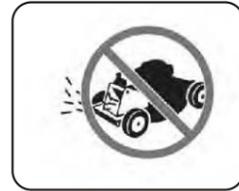
Never operate the lawn mower with discharge chute open
