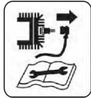
Remove spark plug before maintenance
