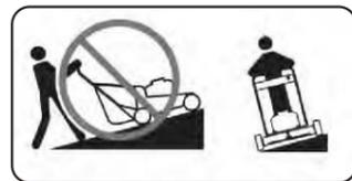
Do not mow excessively steep slopes, mow a cross the face of slopes, never up and down
